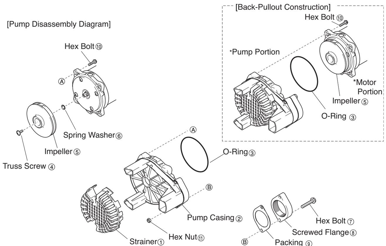
**Note:** The description of the diagram may differ slightly in shape and construction depending on the model.
