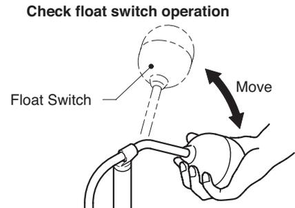
**Note:** Allow the pump to operate a minimum of 2 seconds for each trial operation. The trial operation must be completed within 1 minute.
