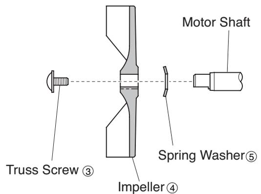
[Assembly direction of spring washer]
