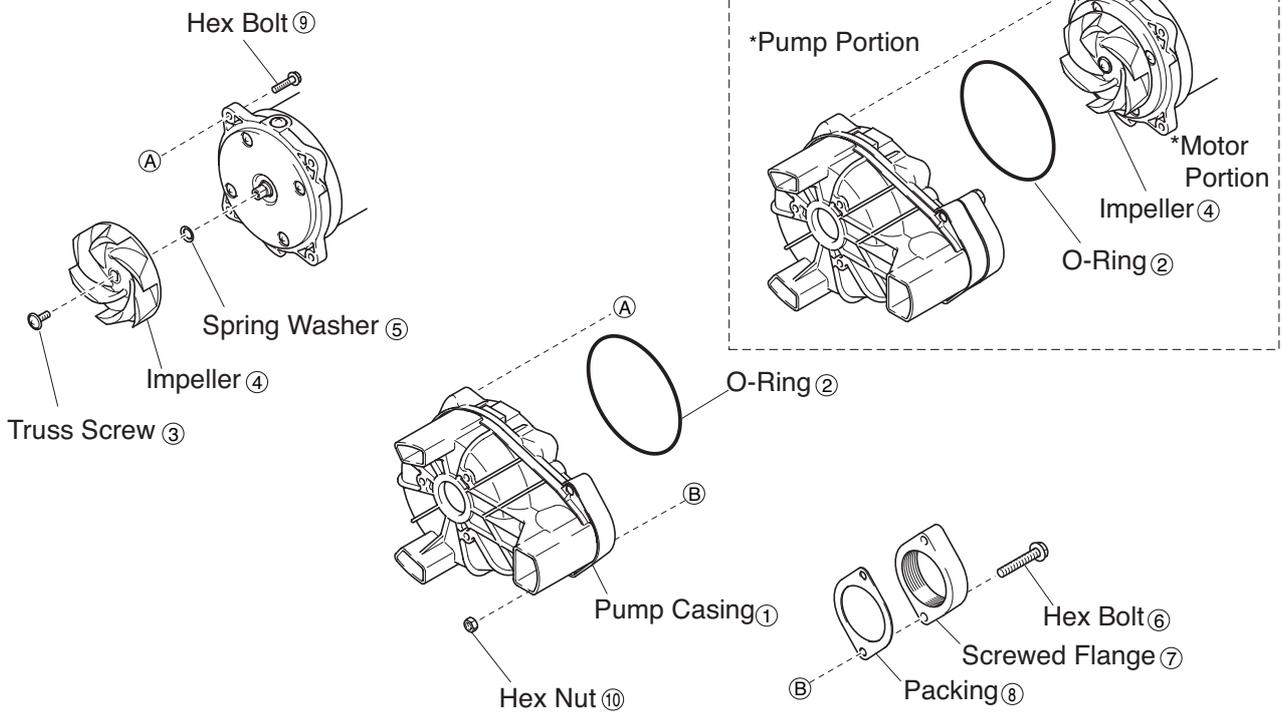
**Note:** The description of the disassembly diagram above may differ slightly in shape and construction depending on the model.
